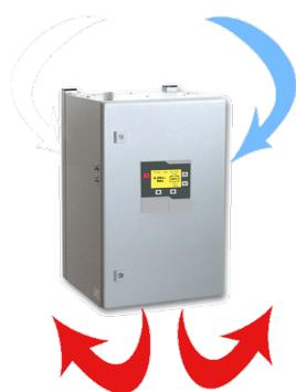
Charger is designed for wall-montage or for stand. Ventilation cold air intake is located on the side of the charger and after cooling HF modules the warm air is taken away from case through vent outlet on the bottom side of the charger. Suction and exhaust are equipped with filters resistant to spraying water and dust nuisance.
